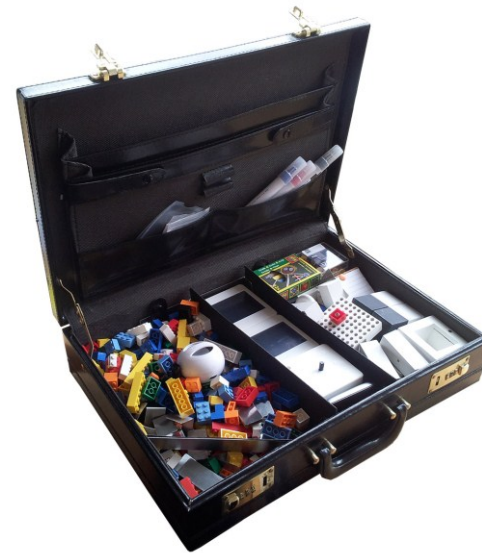
Figure 1: Prototype of Materialise, with the 'active building blocks' in the center and the 'passive building blocks' left and right.
