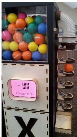
Figure 2. The ball tube at the side of the VoxBox drops the ball through step by step after completing question modules.
