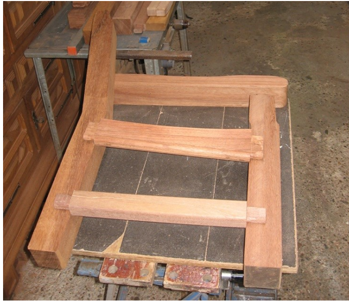
Fig. 4.6 In John's garden bench the wood is connected with pins that slot into other pieces of wood, instead of with screws, because this gives a more beautiful result.
