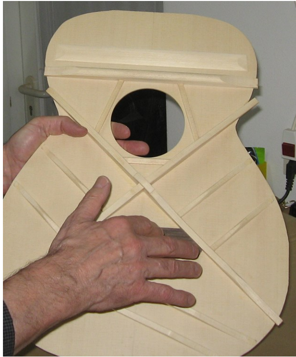
Fig. 4.3 Paul was experimenting with different bracing constructions for the back panel.
