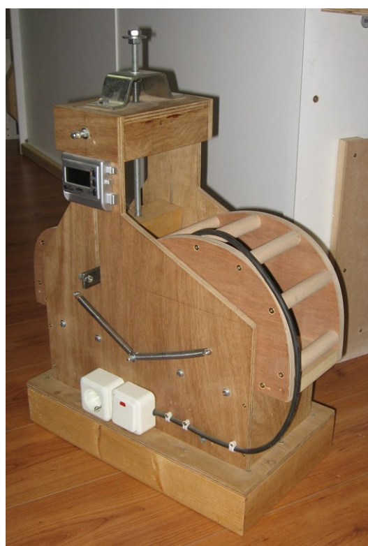
Fig. 4.8 Paul’s self-made electronic tool for bending the thin side panels of the guitar’s belly with the aid of a heating element.
